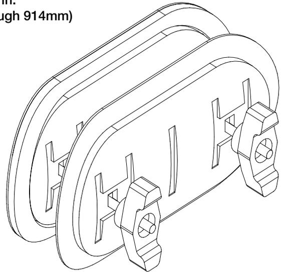
**INSTALLATION:** Easy installation. Self adhesive cut around template is provided for the exact size duct opening required. Cut opening around perimeter of template. Insert door into opening at an angle and tighten knobs (Do not over tighten).
